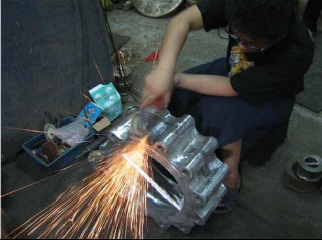
Trimming of die casting parts
